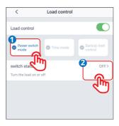
Time mode: set the time to enable/disable the load, and the load will be turned on or off automatically within the setting time period. Select standard mode or intelligent mode based on your actual needs.
